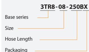
**BC:** continuous length in box**BX:** 2 lengths per box, no length less than 20 ft.**RL:** random length reel, 2 lengths per reel, no length less than 20 ft.**R:** continuous length on reel**3TR8 supersedes**
