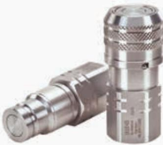
Eaton's MLFF Series stainless steel coupling is a flat face dry break coupling used for hydraulic applications. The MLFF Series interchanges with all ISO 16028 profiles. Due to its stainless steel design, it is corrosion resistant and can handle aggressive environments.
