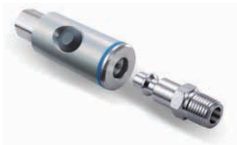
Eaton Gromelle™ ID10900 Series is a single shut-off compressed air coupling that interchanges with ISO 6150 C Standards requirements. Nominal diameter is 8 mm. Thanks to a distinct two-movement action, our couplings guarantee operator safety at disconnection by eliminating the "whiplash" effect. It is a must-have for safe air applications.
