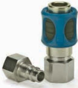
Eaton Gromelle™ G700 Series is a single shut-off compressed air coupling with a European profile. Nominal diameter is 7.2/7.4 mm. This coupling offers an excellent flow capacity and is used in compressed air applications.
