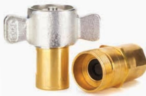
Eaton's 5100 Series brass coupling with steel tubular valve offers minimum air inclusion and fluid loss. Thread together latch provides connect under pressure capability and vibration resistance. The 5100 Series is not rated for continuous hydraulic impulse applications. For hydraulic impulse applications, refer to the FD86 and FD96 Series thread to connect product lines.
