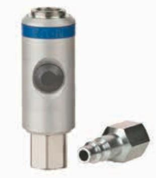
Eaton's Safeline Series is an Industrial Interchange pneumatic coupling with push button safety feature designed for use with compressed air. Two-step disconnect procedure shuts off air supply and releases downstream air pressure before plug can be removed from socket/female, which prevents hose whip.
