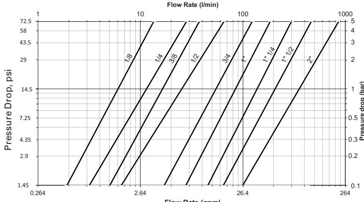
Test Fluid: Oil viscosity 30 cSt at 40°C/104°F
