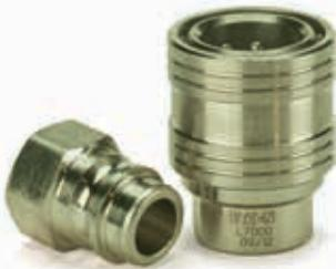
Eaton's L7000 Series brass quick disconnect coupling is a full-flow coupling suited for applications where maximum flow capacity is required and valving is not needed. Mainly used in fluid transfer applications where stainless steel is not a requirement, it can handle a wide range of media and offers good corrosion resistance.
