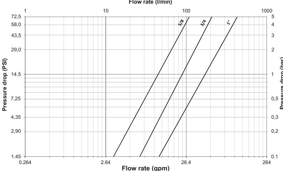
Hydraulic Oil viscosity : 30 Cst at 40°C / 104°F
