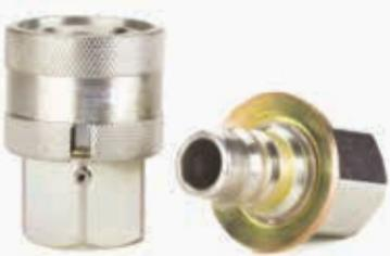
Eaton's FD69 Series design has a greater surface contact area for long service life in rugged high pressure and water blast applications. The maximum operating pressure is 10,000 psi with 40,000 psi minimum burst pressure.
