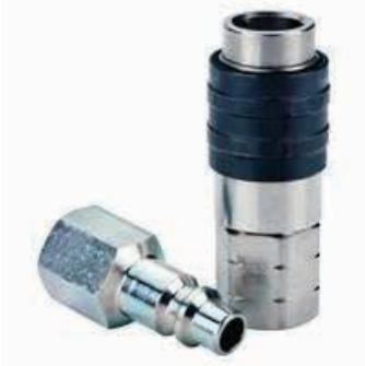
Eaton Gromelle™ I900 Series is a single shut-off compressed air coupling that interchanges with ISO 6150 B and US A-A-59439 Standards requirements. Nominal diameter is 8 mm.
