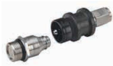
The Eaton FD17 high pressure coupling can be connected by hand while under pressure up to 4,500 psi/310 bar. This quick disconnect coupling is most commonly used in SCBA transfilling and buddy breathing applications and is commonly found on SCBA equipment certified to various NIOSH, NFPA and CBRN standards.
