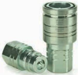
The IA Series meets ISO 7241-1 A Standard requirements and has a push-pull design, which allows the socket to be bulk-head-mounted. This configuration provides automatic connection or disconnection via a simple push or pull of the plug. Our IA Series is available in  $\frac{1}{2}$ " with female or male end connections such as tube fittings, NPT, metric or SAE threads. It is widely used in agriculture and forestry applications.
