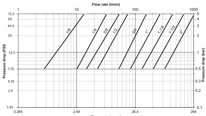
Applicable to valves with 0.5 bar (7.25 psi) cracking pressure
