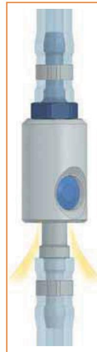
The plug is retained in the socket:
