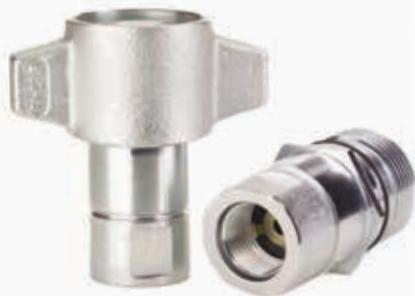
Eaton's FD86 Series is a thread together steel quick coupling offering dry break and high impulse technology and capabilities. The maximum operating pressure is 5,000 psi. The FD86 Series is available in either wing nut or hex nut configurations for ease of assembly and disassembly. (For higher pressure applications and additional size requirements, refer to FD96 on page 44.)
