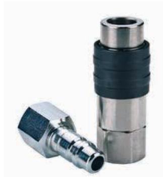
Eaton Gromelle™ T1100 Series is a single shut-off compressed air coupling that interchanges with ISO 6150 B and US A-A-59439 Standards requirements. This coupling offers excellent flow capacity and is used in many compressed air applications.
