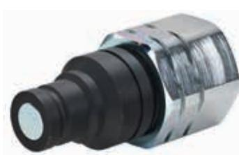
Eaton's FFCUP Series plug/male coupling is an ISO 16028 standard interchange. The flush face design prevents fluid loss on disconnection and air inclusion on connection guaranteeing excellent flow capability. An integrated patented system allows the FFCUP Series plug to be connected to a socket/female half coupling under 350 bar (5075 psi) residual pressure.
