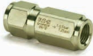
The Eaton R4000 Series brass check-valves are designed to either allow flow of fluid in one direction only or limit the line's internal pressure to the cracking pressure. Standard cracking pressures are 0.5 and 1 bar (7.25 and 14.5 psi). Alternatives can be offered upon request. It is designed to handle liquids in all industries and for fluid transfer lines.
