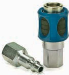
Eaton Gromelle™ G600 Series is a single shut-off compressed air coupling that interchanges with ISO 6150 B and US A-A-59439 Standards requirements. Nominal diameter is 5.5 mm. Its new revamped design and the materials used make it a rugged and long-lasting coupling, offered in a wide selection of end connections. It is used in general pneumatic applications.
