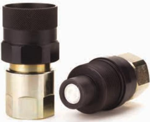
Eaton's FD96 High Pressure Thread Together Flush Face Series is designed for high pressure and high impulse applications for hydraulic circuits. The FD96 Series design provides low connect and disconnect force in hydraulic circuits where trapped residual pressure must be addressed. The flush face design limits contamination and unwanted fluid loss. The FD96 Series is available in sizes 1/4" through 2" to best meet your specific size requirements.
