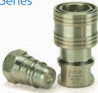
Eaton's H5000 Series brass quick disconnect coupling is a pull-to-connect double shut-off coupling. It is a general purpose industrial quick disconnect coupling with the original Eaton's Gromelle™ profile. Mainly used in fluid transfer applications where stainless steel is not a requirement, it offers a good alternative for corrosion resistance.
