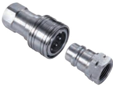
The H15000 Series is a general purpose industrial interchange coupling that meets the ISO 7241-1 Series A standard. The H15000 Series features a rugged ball latch mechanism with self-sealing poppet valves.
