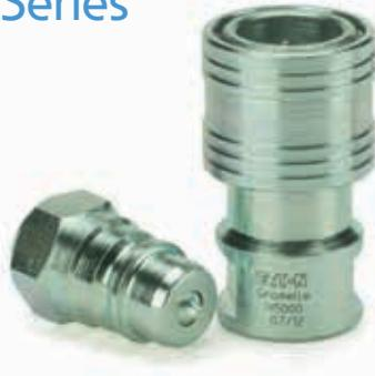
Eaton's H5000 Series steel quick disconnect coupling is a pull to connect double shut-off coupling. Featuring the original Eaton's Gromelle™ profile, it remains as the series users prefer when it comes to severe hydraulic applications such as high pressure, pressure impulses, heavy mechanical loads and frequent connection and disconnection cycles. The unique sleeve lock option offers a reliable solution and benefit to the end user when safety is a concern.
