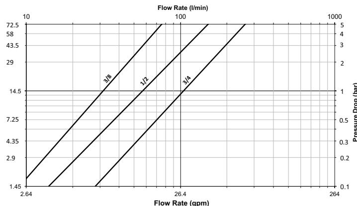
Test Fluid: Oil viscosity 30 cSt at 40°C/104°F
