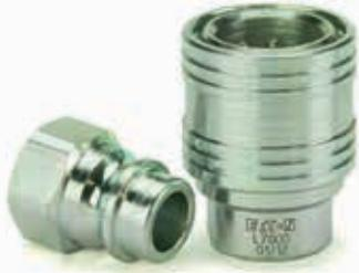
Eaton's L7000 Series steel quick disconnect coupling is a full-flow coupling with a rugged construction. Similarly to Eaton H5000 Series, the heat treatment and hardened materials give the coupling excellent resistance to mechanical and hydraulic demands. It is suited for applications where maximum flow capacity is a requirement and valving is not needed.
