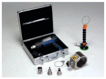
Hand held electric heat gun basic kit (up to 1-1/2" hose ID and tube ends)
